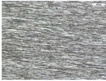
Fig. 3. Microstructure of specimen no. 2, pearlitic steel after cold working, visible 85% material reduction. LM.
